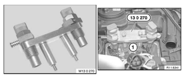
Note: Do not open the high pressure fuel injection system if the coolant temperature is above 40°C. The residual pressure in the high pressure fuel system could cause bodily injury.
